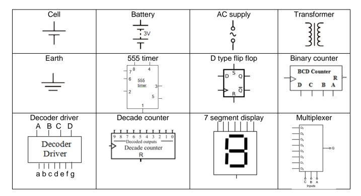
Circles can be put on S and R inputs for D types, and on CK and R inputs for counters (or bars over the letters) when inverted.
