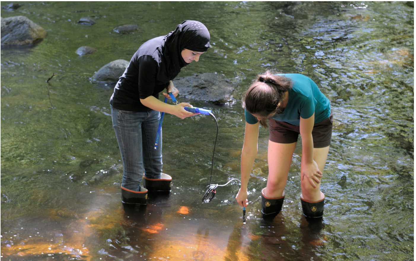
Measuring oxygen using digital oxygen probe Martin Shields / Alamy Stock Photo
