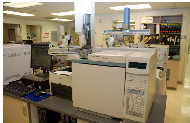
Gas liquid chromatography instrument used in a forensic lab Mikael Karlsson / Alamy Stock Photo
