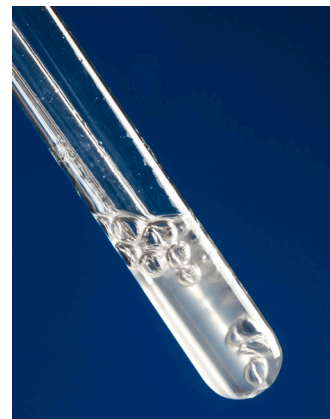
Test for carbonate ion Martyn F. Chillmaid / Science Photo Library
